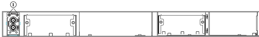
Figure 338: Tighten Screws on the Inserted Clock Module
