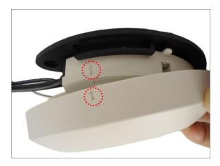
**NOTE:** If the cable(s) will be routed along the ceiling or wall, route the cable(s) through the cable gap of the cover ring.
