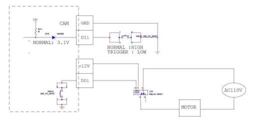
Note that when choosing an appropriate relay, please refer to its specifications and make sure they match the above design. The triggering circuit voltage has to be around 12V DC and the switch-controlled circuit voltage has to match the external power supply (e.g. 110V AC or 220V AC).
