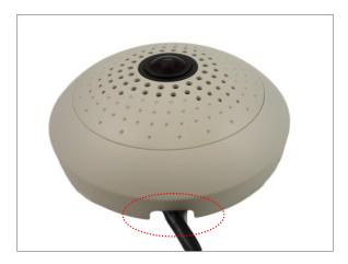
2. Twist the ring counter-clockwise to secure the ring to the camera.
