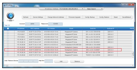
You can quickly notice the camera model in the list. Click on the IP address to automatically launch the default browser of the PC with the IP address of the target camera already filled in the address bar of the browser.
